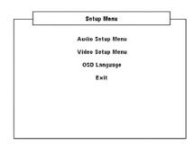
At any source mode, press the HTR 6's [SETUP] button for the Setup Menu OSD to appear. With the use of the HTR 6's navigation buttons, you may select various menus. If the Setup Menu does not appear, check your applicable video connections.
