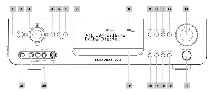
1 POWER BUTTON: Press this button or the HTR 6 remote's [ON] button to switch ON the VISO TWO. The Standby LED indicator will turn from amber to blue and illuminate the VFD. Pressing the power button again or HTR 6's [OFF] button turns the unit back to standby mode.
